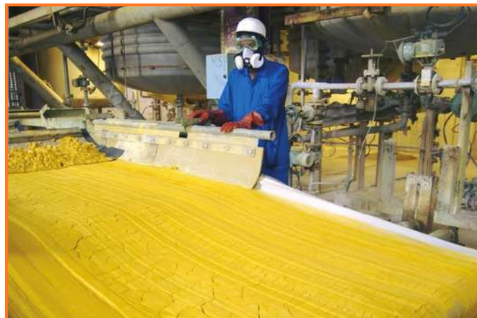
Yellowcake being produced in South Africa for export (also known as urania) is a coarse, powdered uranium ore concentrate that represents an intermediate milestone in the processing of uranium. Containing roughly 70% to 90% uranium oxides (yellowcake is U_3O_8 ), it serves as the global feedstock for nuclear fuel production.
