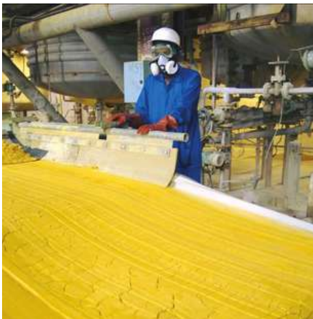
Uranium for export being processed near Johannesburg, This form is known as Yellowcake and is a Uranium Oxide.
