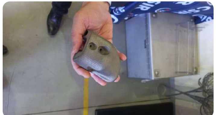
A high strength industrial component produced entirely using Titanium. It was built with a laser, and amazingly, weights about the same as an egg.
