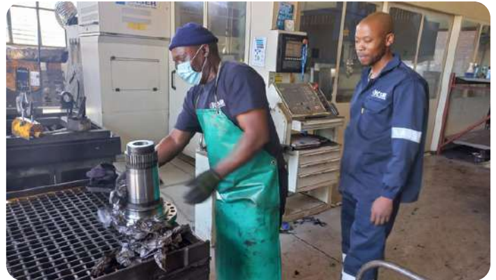
This is a shaft for an industrial customer, which had just been refurbished by means of a laser system. The diameter of the shaft was increased using a laser to lay extra metal onto the outer surface.
