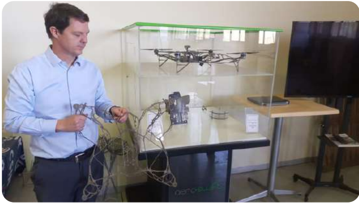
Dr Hencharl Strauss showing the body of a drone created entirely using a laser.
