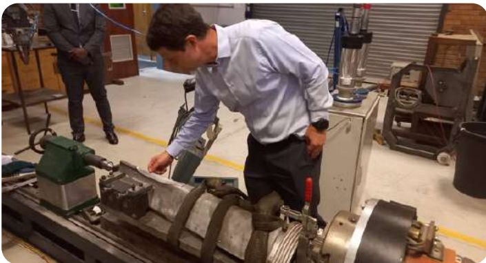
Dr Hencharl Strauss examining the leading edge of an industrial turbine blade, which is being refurbished using a laser system.
