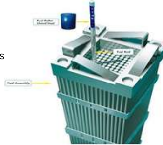
ILLUSTRATION OF A KOEBERG-TYPE FUEL ELEMENT OF 17X17 ZIRCALLOY TUBES 3,4M LONG.
