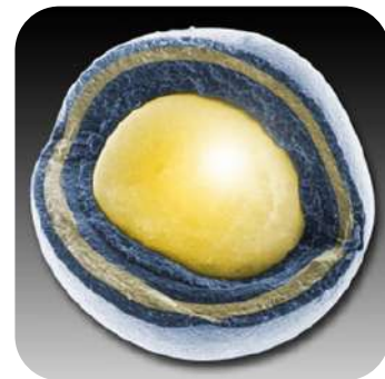
TRISO PARTICLE - NEARLY 1 MM DIAMETER
